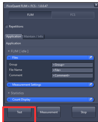
Fig. 2.5: Start a test measurement with the ZEN PicoQuant Application
